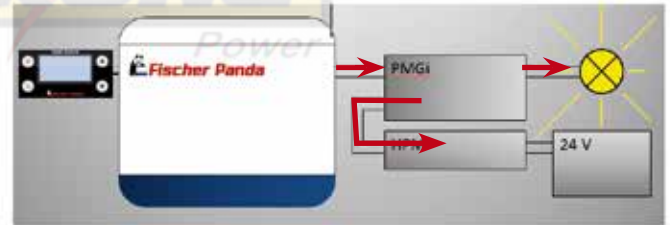
Generator and battery charging: 2-4 kW
