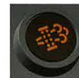
DPF regeneration control panel
