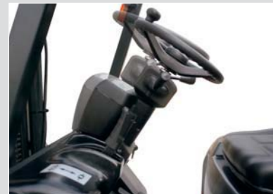
Adjustable Steering Wheel Steering wheel can be adjusted by a lever on the right-hand side for the most comfortable operator position.
