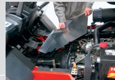
Easily-Detached Floor Panel One-touch removal of the floorboard gets you right to service operations and reduces down-time.
