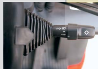
Automobile-Style Light/Turn-Signal Lever The automotive influence seen in the T Series extends to the thoughtful use of an automobile-style light and turn-signal lever, with simple actions that let the operator focus on the job.
